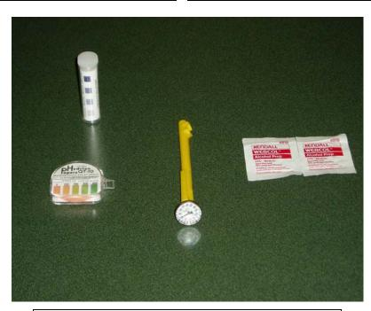
SANITIZER TEST STRIPS, 0-220 °F METAL STEMMED THERMOMETER & ALCOHOL SWABS FOR CLEANING
