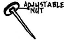
To correct an inaccurate thermometer:
